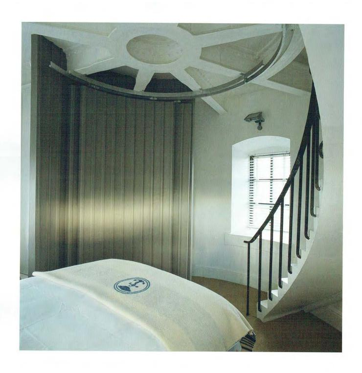
Above: in the adults' bedroom on the second floor, a curved track is mounted to the underside of the original riveted steel beams to allow sections of curved wall to be drawn across for privacy from stair traffic. The staircase leads to the library and above that is the lantern room. Opposite: the bed is laid with monogrammed linen from The Plaza hotel in New York and an Italian naval blanket. The picture of a unicorn is by Mark Wallinger
