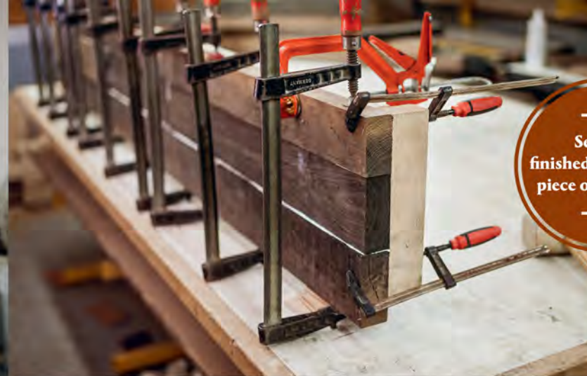
Day 9: Creation of the end grain blocks ready for tapering
