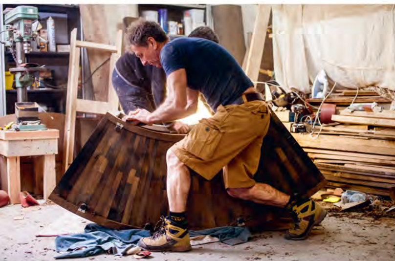
Day 19: On to the fifth and final grade of hand sanding
